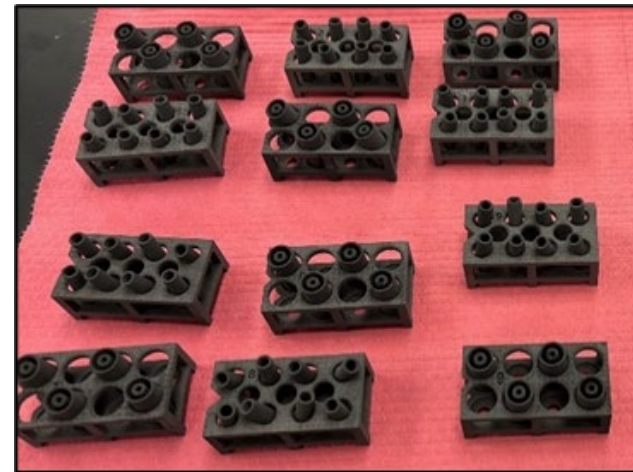
Development Carbon pellet preforms loaded onto tooling racks for insertion into BWXT's CVI furnace
