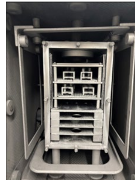
BWXT CVI furnace retort loaded with carbon matrix HALEU specimens.
