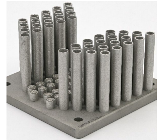
Rabbit capsules—small sample holding devices—are the first pressure-retaining components printed and installed in HFIR
