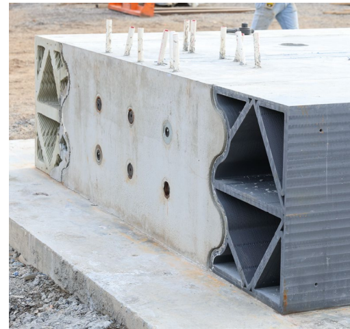
Large format polymer printing technology industrially commercialized for nuclear infrastructure
