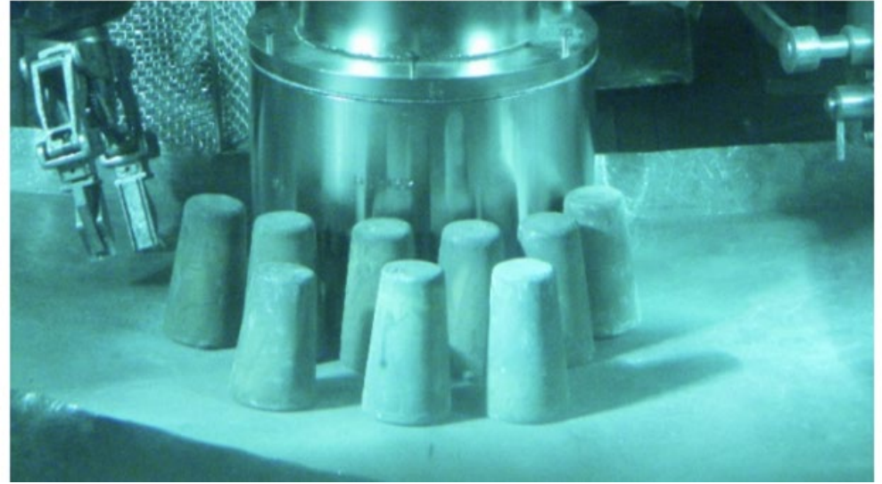
HALEU reguli produced from recovered EBR-II fuel
