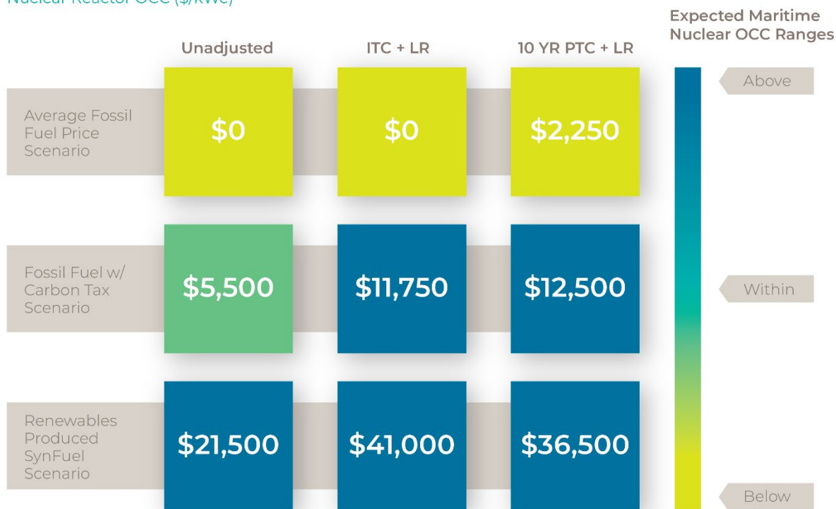
Figure 1. Breakeven nuclear plant OCC diagram for synthetic maritime fuel production.
