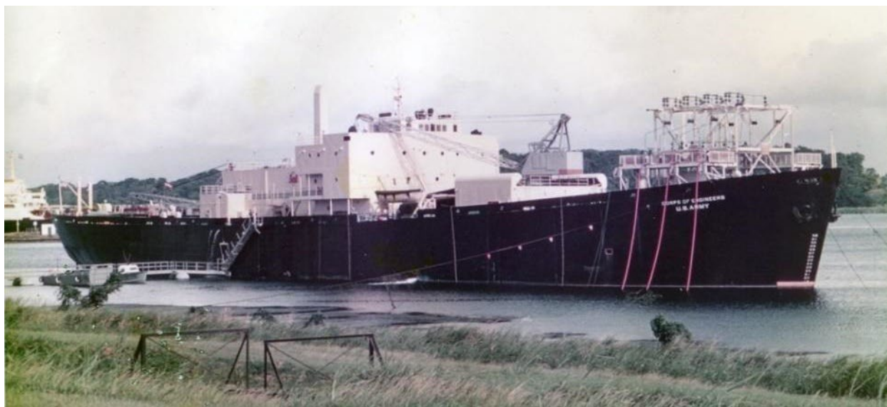
Figure 21: STURGIS operating in the Panama Canal Zone. The Sturgis, a former World War II Liberty Ship, was converted into the first floating nuclear power plant in the 1960s [42].
