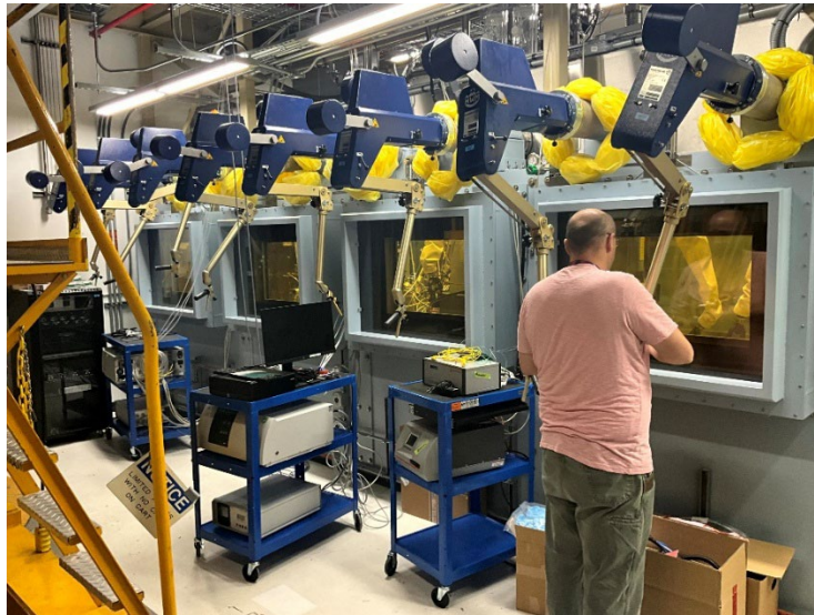
Figure 22: MSTEC Project Team Testing Telemanipulator Operation
