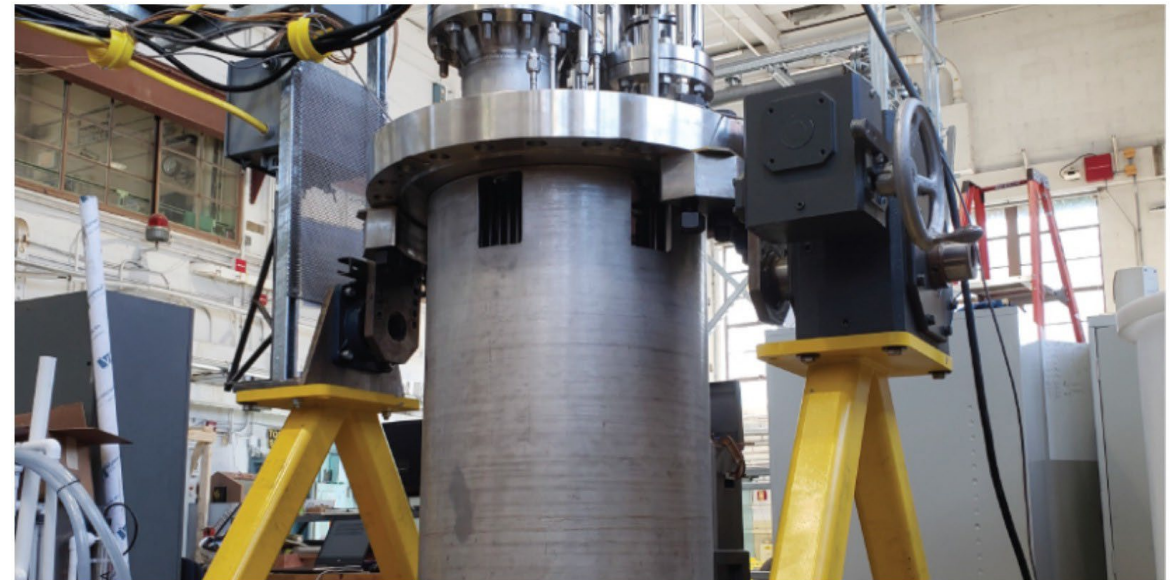
The primary system of THETA at Argonne's Mechanisms Engineering Test Loop Facility, where Oklo is conducting sodium thermal-hydraulic testing with support from a GAIN award announced in 2021. (Image: Argonne National Laboratory)
