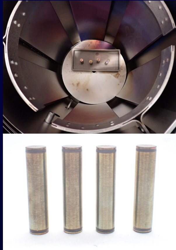
Moderator Canning Demonstration and Hydrogen Dissociation Measurement
