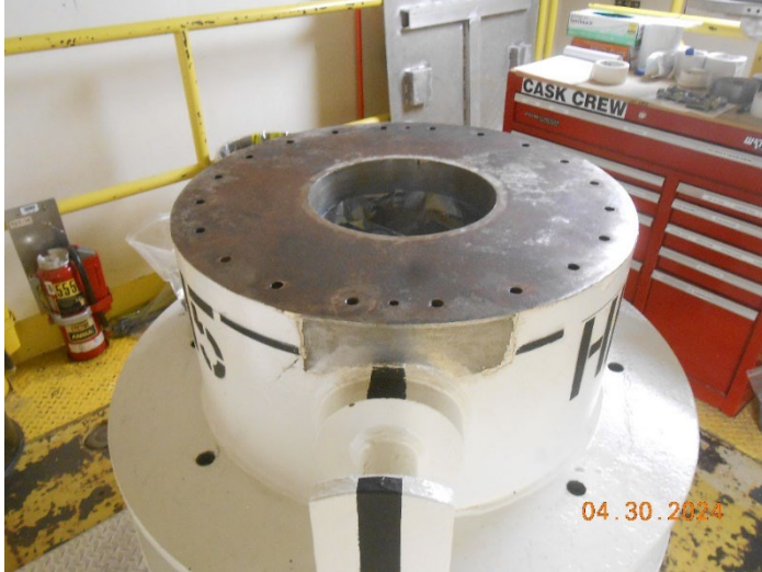
Figure 25 The disassembled and cleaned HFEF-15 cask body.
