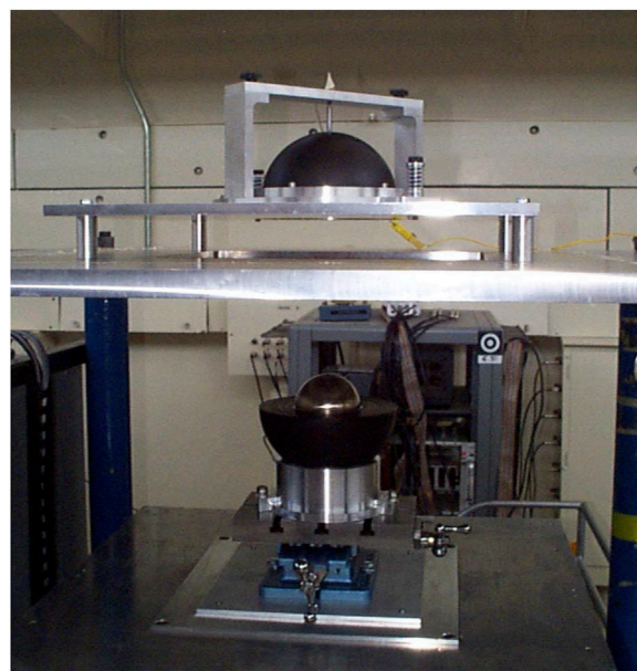
FIGURE 12 Np sphere with highly enriched uranium shells mounted in the planet assembly.
