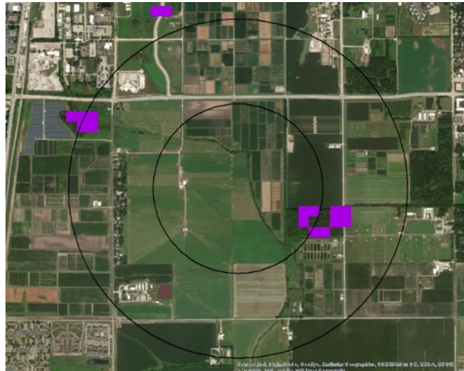
Figure 6-65: The UIUC Search Area OR-SAGE results for wetlands and open water indicates limited site impact beyond the central site area.
