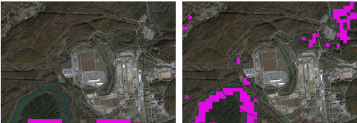
Figure 6-53: The ETTP OR-SAGE results for floodplains (left) and wetlands and open water (right) indicates limited site impact beyond the central site area.
