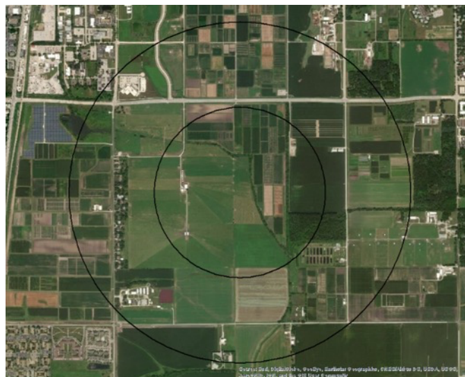
Figure 6-64: UIUC Search Area OR-SAGE results for faults, safe shutdown earthquake, slope, 100-year floodplain, protected lands, and landslide risk indicate no query threshold issues.
