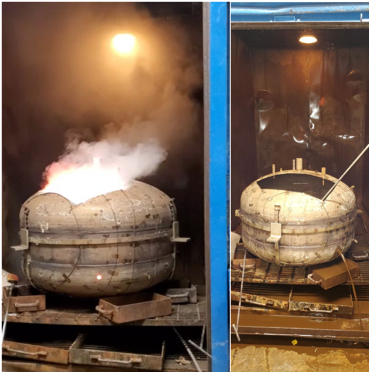
Figure 28. Legacy Dump Tank Contents on Fire (left) and Rinsing Dump Tank with Water Post-Burn (right).
