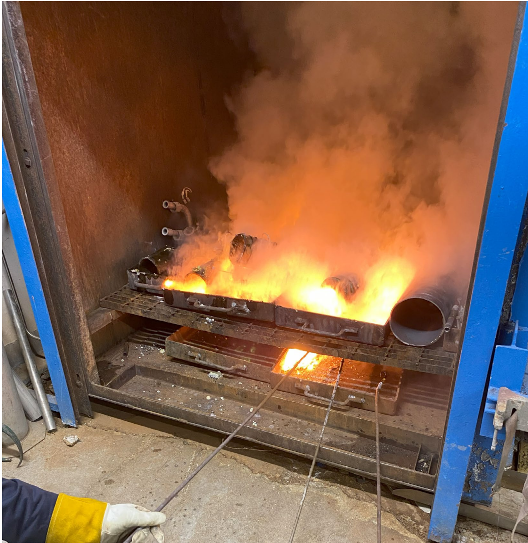
Figure 29. Various Sodium Service Components on Fire.
