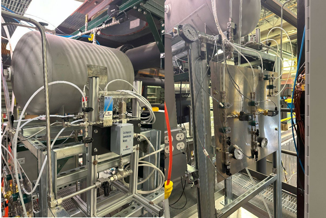
Figure 19. Nitrogen gas and water vapor mixing system (left) and gas supply manifold (right).
