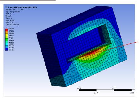
Steady-state concrete temperatures from preliminary design
