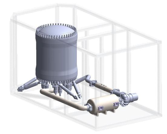
Reactor Core, Pressure Vessel and Primary Loop
