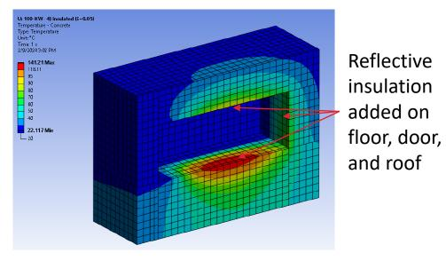
Steady-state concrete temperatures from conceptual design
