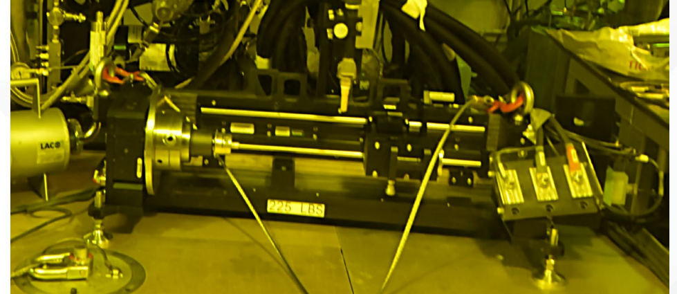
Above: one of two new welding systems installed to perform fuel refabrication in HFEF.
