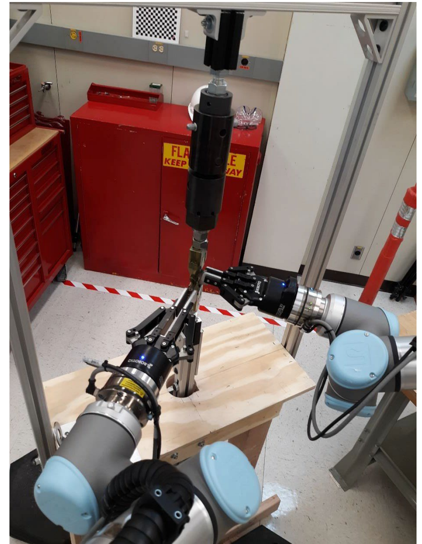
Loading \frac{1}{2} compact tension specimen in Instron mockup via two UR10E robots
