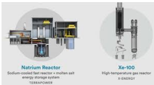
Figure C3.3. Schematic of Natrium metal-fueled SFR concept and Xe-100 HTR TRISO-fueled concept funded by DOE-NE.
