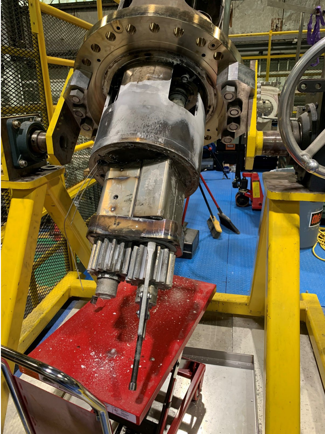
Figure 7 - Gear Test Assembly - in process of being disassembled following carbonation process. The white powder is sodium bicarbonate – the reaction product of the carbonation process.
